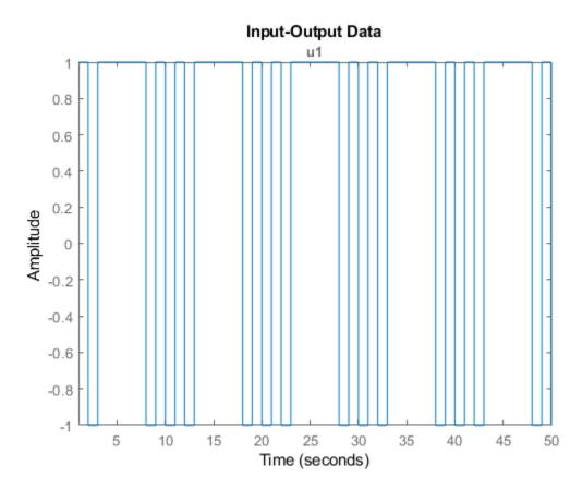
As specified, the generated single-channel periodic random binary input signal has a period of 10 seconds, and there are 5 whole periods in the signal.
