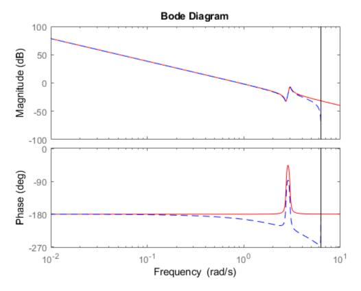
The first PlotStyle, 'r', specifies a solid red line for the response of H. The second PlotStyle, 'b--', specifies a dashed blue line for the response of Hd.
