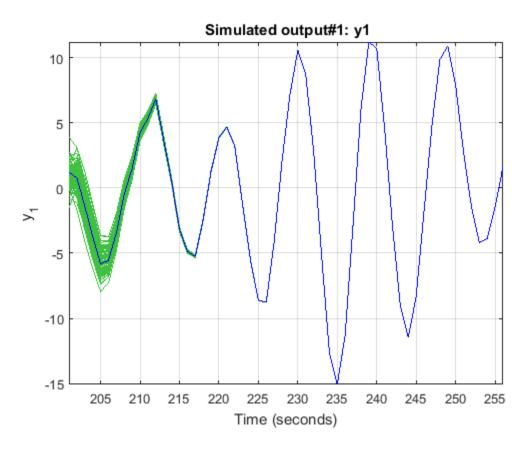
The blue line plots the simulated response of the original nominal model sys. The green lines plot the simulated response of the 100 perturbed realizations of sys. The software uses a different realization of the initial states to simulate each perturbed model. Initial states are drawn from a Gaussian distribution with mean InitialCondition and covariance X0Covariance.
