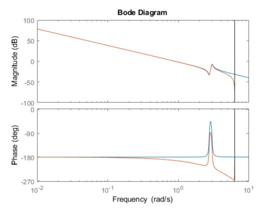
The Bode plot of a discrete-time system includes a vertical line marking the Nyquist frequency of the system.
