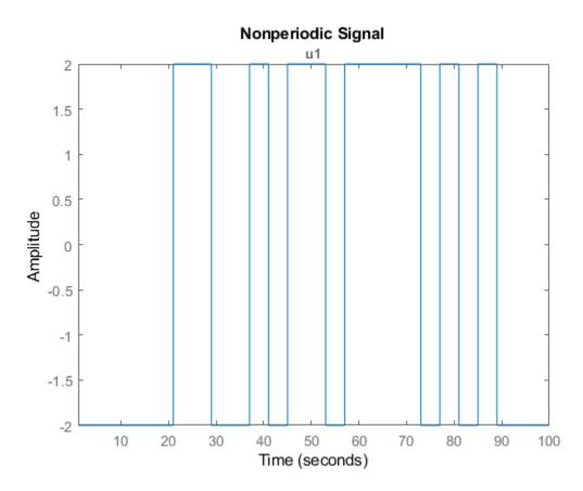
The generated signal is a nonperiodic PRBS of length 100. The signal remains constant for at least 4 samples before each change in value. Thus, the signal satisfies the clock period specified in Band.
