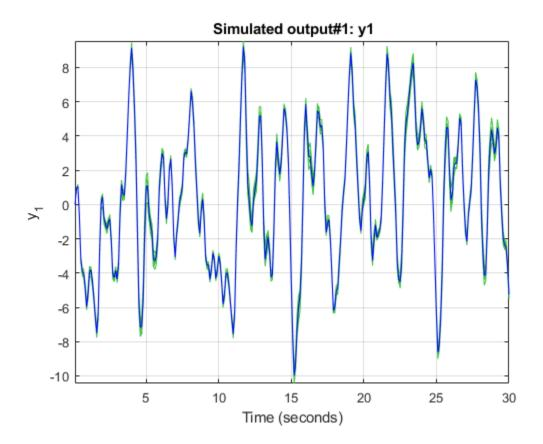
The blue line plots the simulated response of the original nominal model sys. The green lines plot the simulated response of 10 perturbed realizations of sys.
