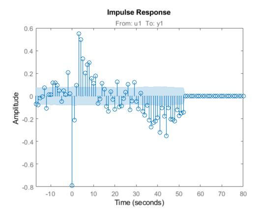
The large response value at t=0 (zero lag) suggests that the data comes from a process containing feedthrough. That is, the input affects the output instantaneously. There could also be a direct feedback effect (proportional control without some delay that u(t) is determined partly by y(t)).
