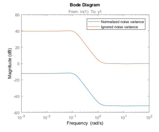
The difference between the bode magnitudes of the noise\_model\_innovation and noise\_model\_normalized is approximately  $51\ dB$ . As expected, the magnitude difference is approximately equal to  $20*log10\ (L)$ .
