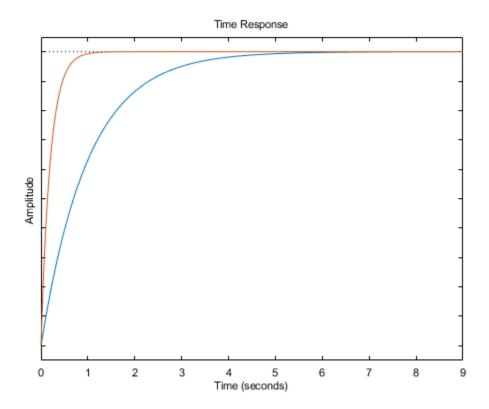
The plot shows the normalized step response for the two transfer function models.
