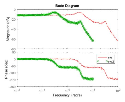
Changing the FrequencyUnit property changes the system behavior. Therefore, the Bode responses of sys and sys2 do not match. For example, the original corner frequency at about 2 rad/s changes to approximately 2 rpm (or 0.2 rad/s).
