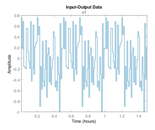
The signal u is generated using 10 sinusoids and has a period of 0.5 hours and 3 periods.
