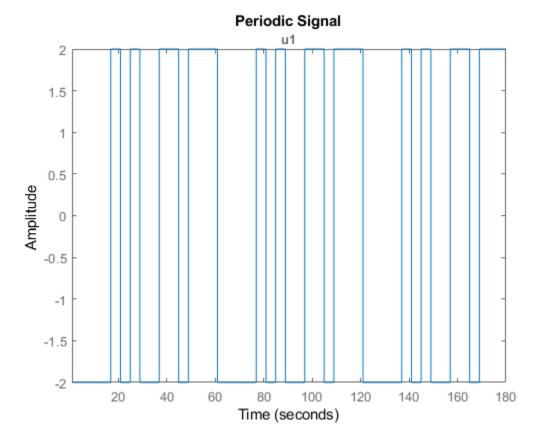
The generated signal is a periodic PRBS with a 60-second period and 3 periods. The signal remains constant for at least 4 samples before each change in value. Thus, the signal satisfies the specified clock period.
