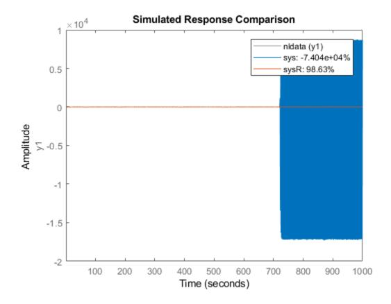
The large negative fit result for the unregularized model indicates a poor fit to the data. Estimating a regularized model produces a significantly better result.
