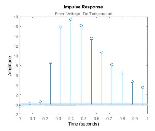
The first significantly nonzero response value occurs at 0.24 seconds, or, the third lag. This implies that the transport delay is 3 samples. To generate a model where the 3-sample delay is imposed, set the transport delay to 3:
