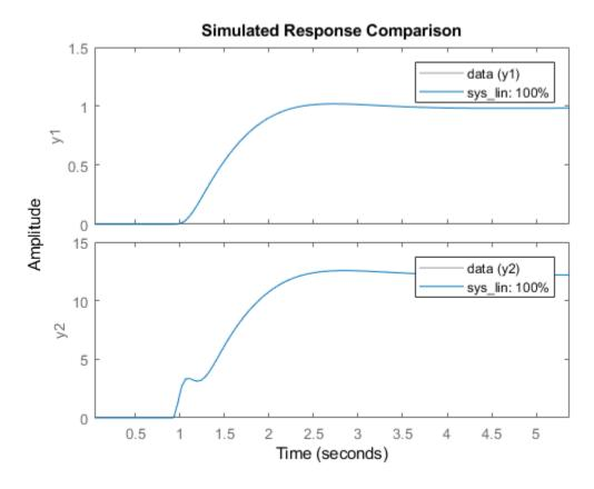
Because the data was obtained by simulating the linearized model, there is a 100% match between the data and model linearization response.
