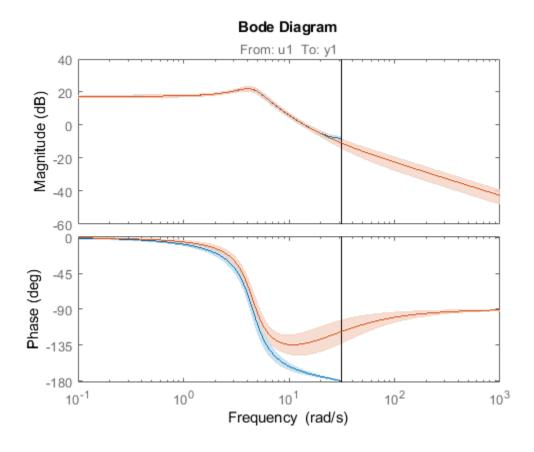
The uncertainties of sys1c and sysd are comparable up to the Nyquist frequency. However, sys1c exhibits large uncertainty in the frequency range for which the estimation data does not provide any information.
