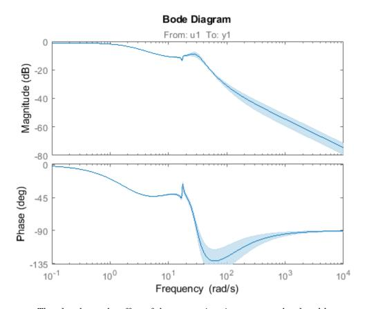
The plot shows the effect of the uncertainty in Plant on the closed-loop response.
