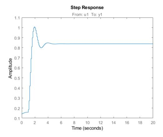
The step response is a steady-state value of 0.8383 at T = 20 seconds.
