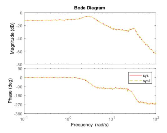
The magnitude and phase of sys and sys1 match because chgFreqUnit command changes the units of frequency points in sys without modifying system behavior.
