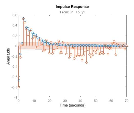
The uncertainty in the computed response is reduced at larger lags for the model using regularization. Regularization decreases variance at the price of some bias. The tuning of the regularization is such that the bias is dominated by the variance error though.
