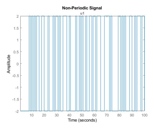
The generated signal is a nonperiodic PRBS of length 100 that switches between -2 and 2.
