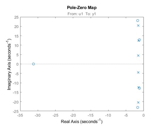
The plot shows that there are two pole-zero pairs that almost overlap, which hints are their potential redundancy.
