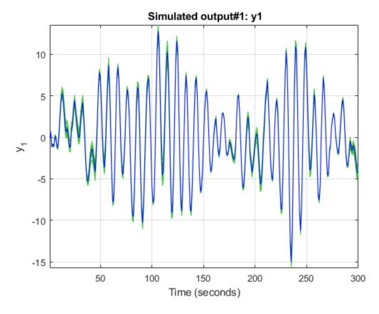
The blue line plots the simulated response of the original nominal model sys. The green lines plot the simulated response of the 20 perturbed realizations of sys.
