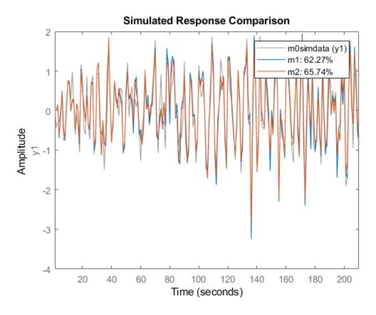
The regularized model, m2, produces a better fit than the unregularized model, m1.
