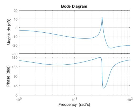
The cell array {1,100} specifies the minimum and maximum frequency values in the Bode plot. When you provide frequency bounds in this way, the function selects intermediate points for frequency response data.
