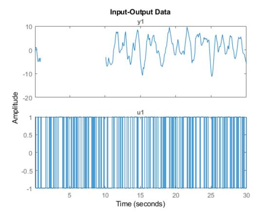
The output data contains missing data between indices 10 and 100.
