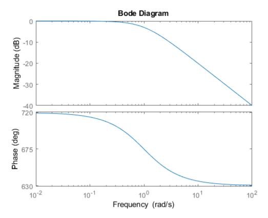
The first bode plot has a phase of -45 degrees at a frequency of 1 rad/s. Setting the phase matching options so that at 1 rad/s the phase is near 750 degrees yields the second Bode plot. Note that, however, the phase can only be -45 + N\*360, where N is an integer, and so the plot is set to the nearest allowable phase, namely 675 degrees (or 2\*360 - 45 = 675).
