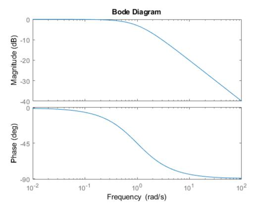
Fix the phase at 1 rad/s to 750 degrees. To do so, get the plot properties. Then alter the properties PhaseMatchingFreq and PhaseMatchingValue to match a phase to a specified frequency.
