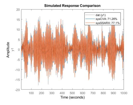
From the plot, you see that the model estimated using the SSARX algorithm produces a better fit than the CVA algorithm.
