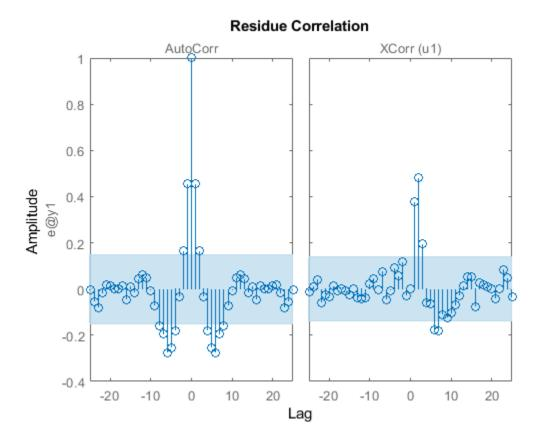
The correlations are calculated until the default maximum lag, 25. The 99% confidence region marking statistically insignificant correlations displays as a shaded region around the X-axis.
