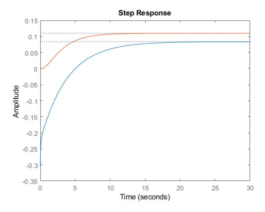
Each step response settles at a different steady-state value. Use the plot handle to normalize the plotted response.
