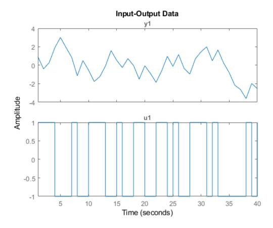
This data contains a change in time delay from 2 to 1, which is difficult to detect by examining the data.
