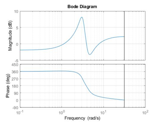
The plot confirms that the maximum gain is approximately 8 dB and the gain peaks at approximately 3 rad/sec.
