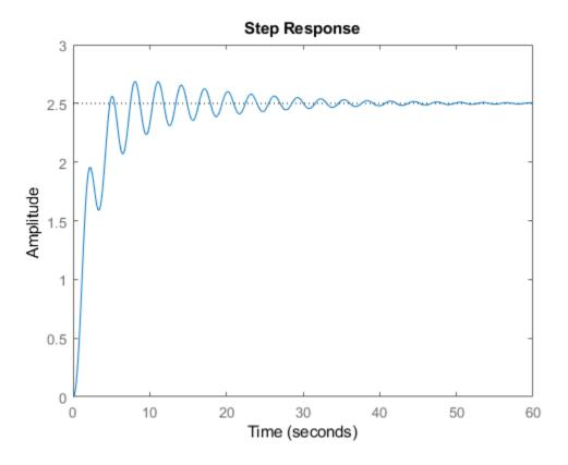
The plot shows that the response rises in a few seconds, and then rings down to a steady-state value of about 2.5. Compute the characteristics of this response using stepinfo.
