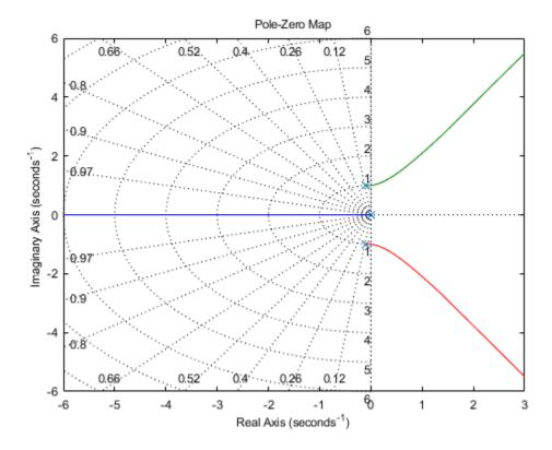
The root locus plot is generated with the grid enabled.
