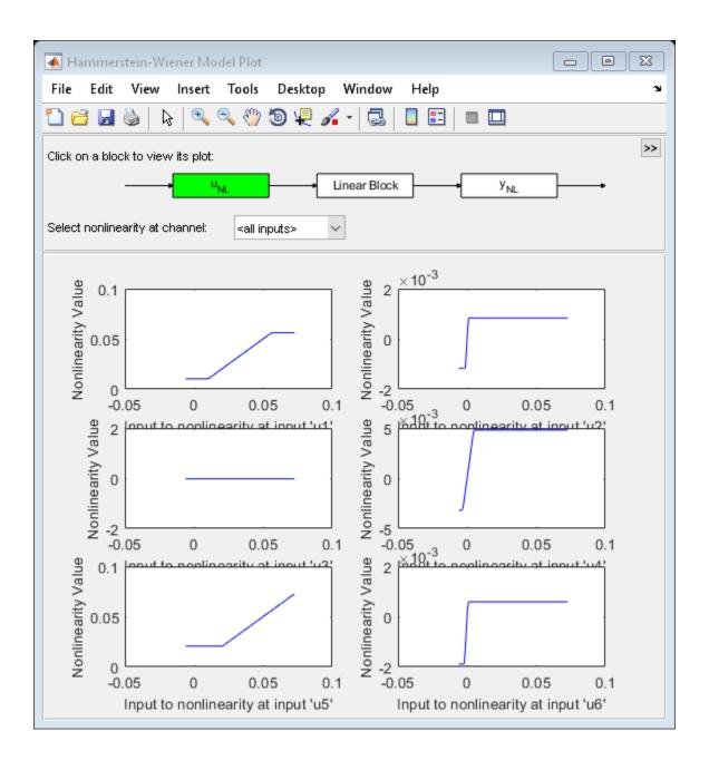
Click on the input and output nonlinearity blocks on the top of the plot to see the nonlinearites.
