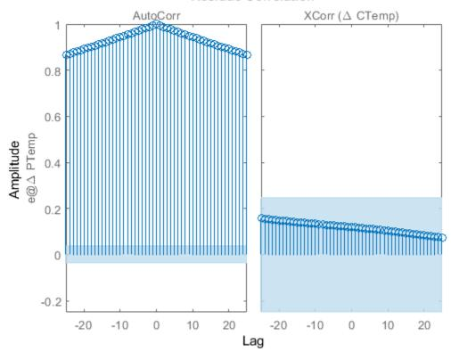
The figure shows that the residuals are correlated. To account for that, add a first order ARMA disturbance component to the process model.
