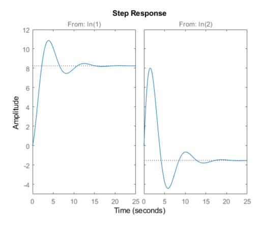
The left plot shows the step response of the first input channel, and the right plot shows the step response of the second input channel.
