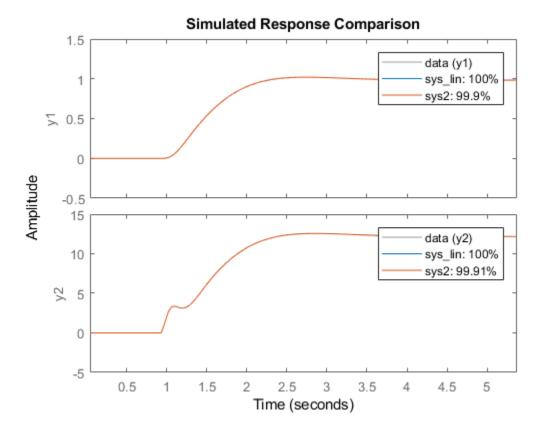
$\tt sys2$  provides a 99% fit for the first output and a 98% fit for the second output while using 4 less states than  $\tt sys\_lin$  .
