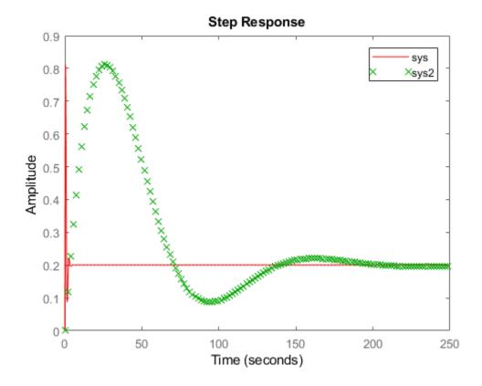
The step responses of sys and sys2 do not match. For example, the original rise time of 0.04 seconds changes to 0.04 minutes.
