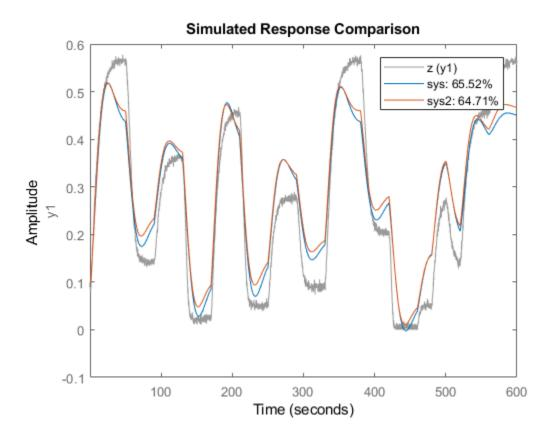
where sys2 refines the parameters of sys to improve the fit to data.
