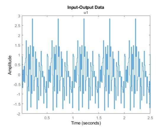
The plot shows that u contains a random segment of 50 samples, repeated 5 times. The signal is a Gaussian white noise signal with zero mean and variance one.
